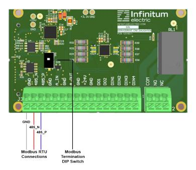
Note: The last unit a daisy-chain configuration should have the Modbus Termination DIP switch "ON". All other units must have the DIP switch in the "OFF" position.
